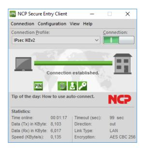
Even if the access point or the IP address changes, Wi-Fi roaming or IPsec roaming maintains the VPN connection. Even behind firewalls whose settings always block IPsec data connections, the NCP Path Finder Technology\* ensures remote access is available.
